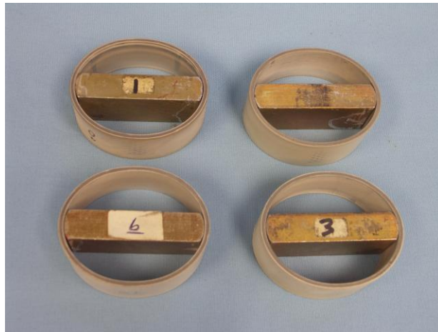
Figure 1 Tin-zinc alloy plated 2a rings with stress bars inserted
