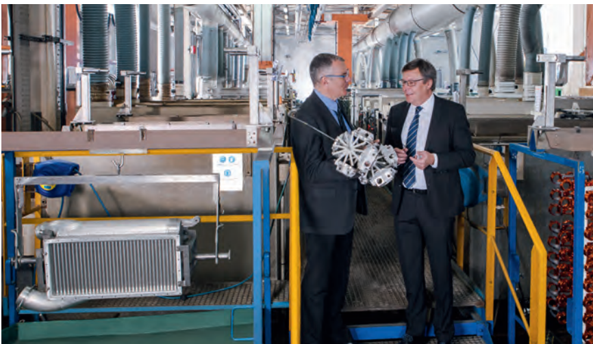
IVD aluminium coating plant in Nottingham, England. Here, Acorn Surface Technology offers a broad spectrum of functional coatings for components in the aerospace industry.
