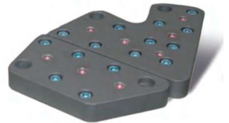
Titanium fittings and titanium pins located near the infrared beam path on the telescope structure. To minimise light scatter, they are provided with a deep black, light resistant, oxide ceramic coating (KEPLA-COAT® black).
