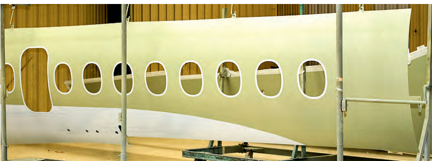
The SKIN PANEL of a FALCON, chromic acid anodised and painted.
