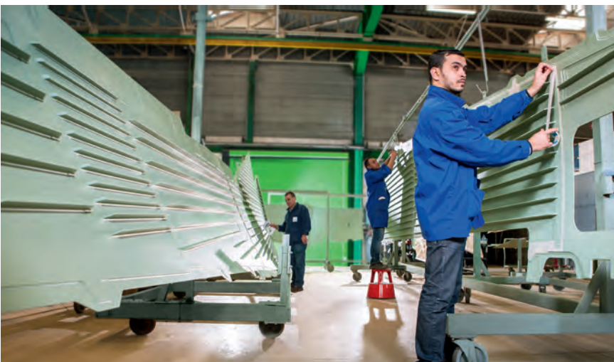
On the left, an aircraft wing is checked before delivery, whilst on the right a wing component is masked for application of a top coat.
