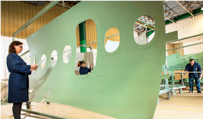
A fuselage panel is checked (left), while behind, wing and structural components are masked for painting.
