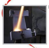
A thermally sprayed coating is applied to improve temperature resistance
