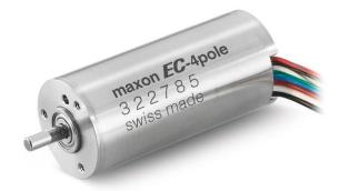
The brushless EC-4pole 22 used in Andy is a true powerhouse. The rotor has two pole pairs for very high power density and high torque. The motor is combined with the planetary gearhead GP 32 HD, which was developed specifically for use under harsh environmental conditions. On the left: the compact assembled drive unit. Image ©Carnegie Mellon University
